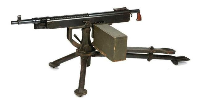
The **Colt-Browning M1895**, nicknamed "potato digger" because of its unusual operating mechanism, is an air-cooled, belt-fed, gas-operated machine gun that fires from a closed bolt with a cyclic rate of 450 rounds per minute. Based on a John Browning and Matthew S. Browning design dating to 1889, it was the first successful gas-operated machine gun to enter service.
